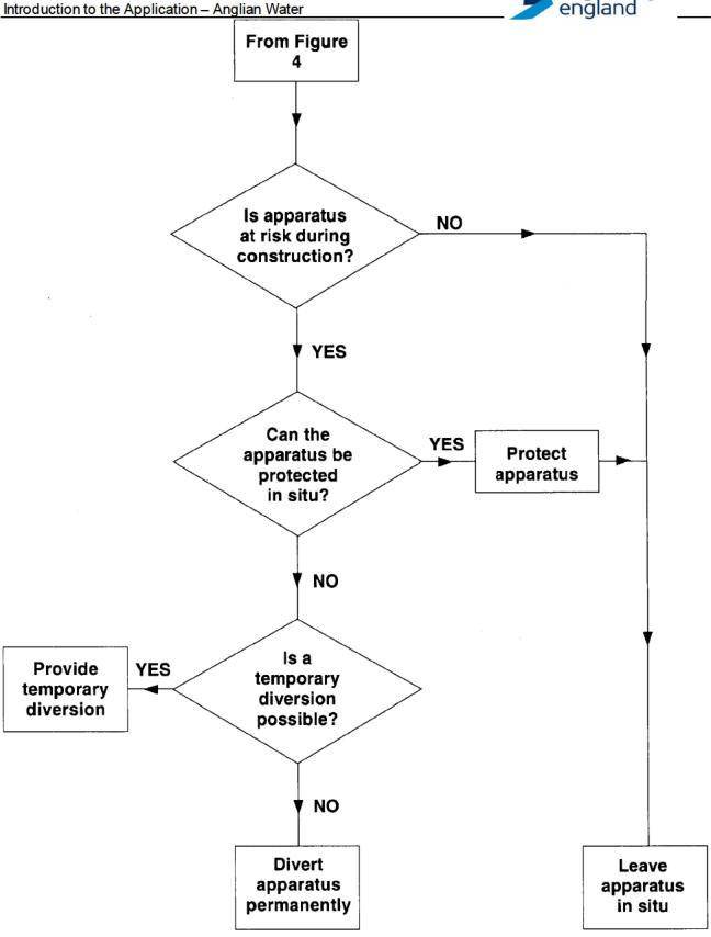
FIGURE 3 APPARATUS AT RISK DURING CONSTRUCTION
